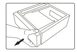
3 **⇒ Drive cage** Loose 2 screws; lift cage up
