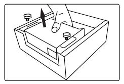
4 **⇒ Remove Support Bar** Loose 1 screw; lift bar up
