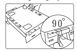
10 **⇒ 5.25"ODD Assembly**Fix drive by M3 screws
