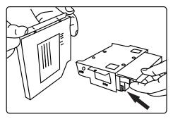
8 **⇒ About cage A**Loose screws and separate cage A and cage B
