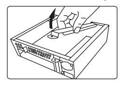
5 **⇒ MB and Add-in-card** Insert I/O shield; fix M/B by 6#32 screws
