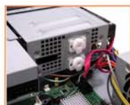
Screwless HDD,ODD FDD assembly (standard devices)
