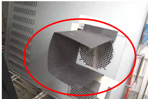
The view of hand made air duct part 2 (Mode 8), the main purpose of this air duct, is to make sure the airflow passed CPU could be exhaust out directly.
