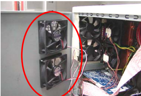
The view of system 9 cm Fan*2(Airflow in).
