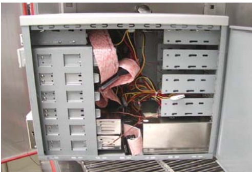
The view of system setup(HDD,SCSI HDD,CDROM,FDD,POWER).
