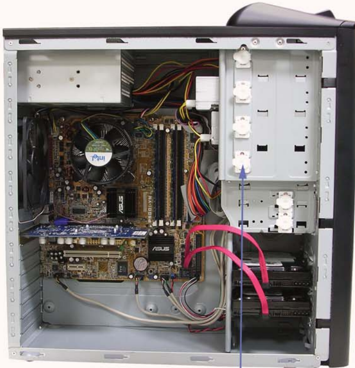
Quick fastener for devices install Screw-less
